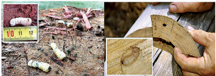
Left: Native longicorn beetle larvae, extracted from jarrah timber. Right: EHB larvae and a cross section of seasoned (dry) pine log showing larvae feeding tunnel.
