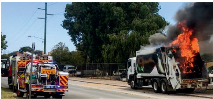
Lithium batteries are a common cause of fires in waste vehicles throughout WA. Picture: City of Swan
